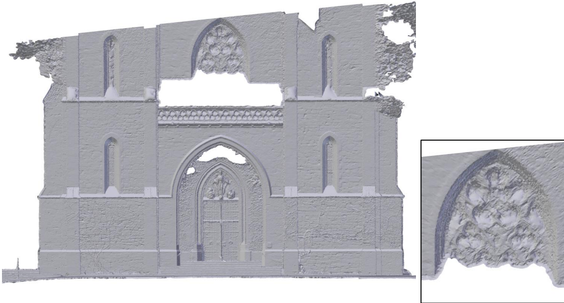
Figure 6: Visible occlusions (holes) in terrestrial laser scan data; (left) artefacts on glass windows
