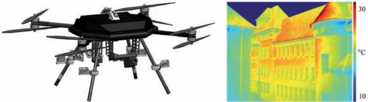
Figure 3: (left) CAD model of an octocopter UAV sensor platform equipped with a thermal imaging camera (right) false-color thermal image of 640 pixels \times 512 pixels. Source: (Patrick Westfeld, 2015)
