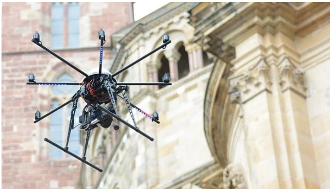
Figure 1: Octocopter 6S12 with mounted camera Sony alpha 7R for photogrammetric measurements
