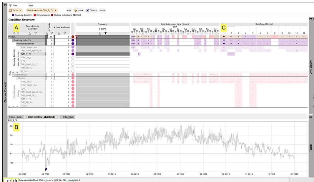
Figure 3. Anomaly and completeness monitor: (A) an instant overview of detected instances that are considered to be an anomaly (in this case outliers), (B) also mapped in purple color in the line plot (illustrated for temperature time series), and (C) over months (for all parameters).
