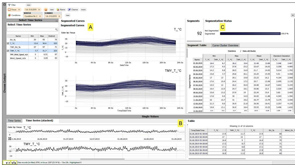
Figure 9. Pattern search and comparison representative of summer period: (A) diurnal summertime temperature distribution; (B) temporal distribution of time series; (C) tabular overview of statistical metrics.
