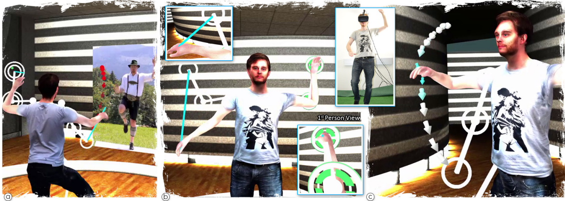
Figure 1.4: Comparing points of view for effective visual guidance. (a) We present motion instructions using the AR mirror visualization technique. We use a split-screen setup on the AR mirror providing a top-down and front view. (b) We provide visual instructions for key poses and motions between these poses. In this example, we show body instructions using a simple stick-figure for key poses. (c) 3D motions are visualized by the corresponding 3D path using a set of 3D arrows. (d) We used a virtual setup to provide the user with a large field of view in all conditions.
