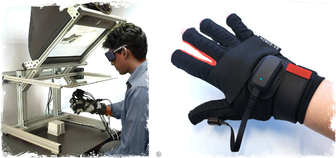
Figure 2.6: Interaction with AR content. (a) Grasping virtual objects with instrumented gloves. Figure adapted from [19]. (b) ManoMotion VR glove with multiple bend sensors for each finger. The rotation of the wrist is tracked with a gyro / accelerometer combination.
