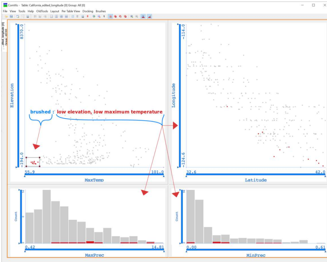
Figure 1.1: ComVis [MFGH08] a coordinated multiple views system is used to analyze meteorology data. ComVis links all its views, when a subset of the brushed data changes in the brushed view. In the shown example, a brush is created in the top-left view and the graphical representation of the data is immediately updated in all other views.
